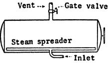
Specifications: A  $2\frac{1}{2}$ -inch vent equipped with a  $2\frac{1}{2}$ -inch gate or plug cock valve and located within 2 feet of the center of the retort.
