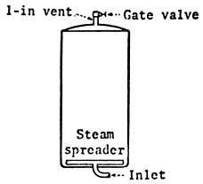
*Specifications*. A 1-inch vent in lid or top side, equipped with a 1-inch gate or plug cock valve and discharging directly into the atmosphere or to a manifold header.
