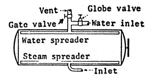
(1) Size of vent and vent valve. For retorts less than 15 feet (4.6 meters) in length, 2 inches (5.1 centimeters); for retorts 15 feet
