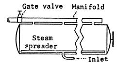
Specifications. One 1-inch vent for every 5 feet of retort length; and vents not over  $2\frac{1}{2}$  feet from ends of retort: Size of manifold—for retorts less than 15 feet in length,  $2\frac{1}{2}$  inches; for retorts 15 feet and over in length, 3 inches.
