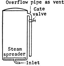
Specifications. A 1½-inch overflow pipe equipped with a 1½-inch gate or plug cock valve and with not more than 6 feet of 1½inch pipe beyond the valve before break to the atmosphere or to a manifold header.
