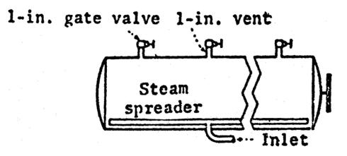
(1) Specifications. One 1-inch (2.5 centimeters) vent for every 5 feet (1.5 meters) of retort length equipped with a gate or plug cock valve and discharging to atmosphere; end vents not more than 2.5 feet (76 centimeters) from ends of retort.
